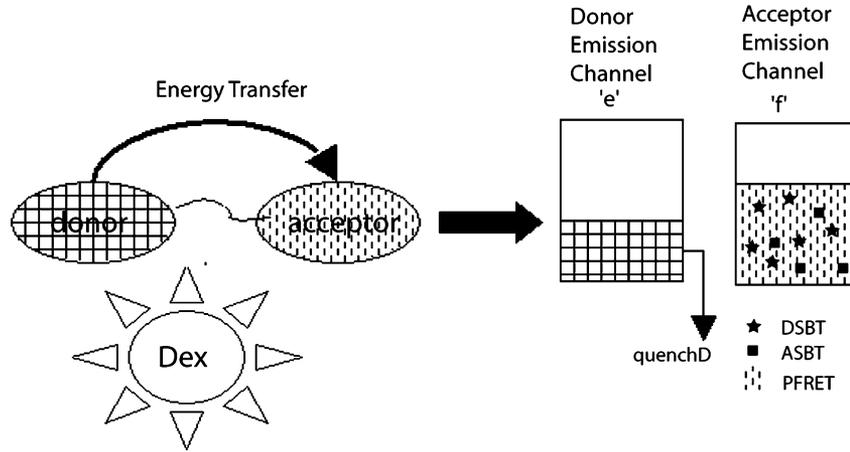
**Fig. 2.** Illustration of DSBT and ASBT signal distribution in the FRET channel. The doubly expressed (labeled) cell excited with donor excitation wavelength the energy is transferred nonradiatively to the acceptor molecules. The energy transferred signal (FRET) detected in the acceptor emission channel ('f') is contaminated with donor spectral bleedthrough (DSBT) and acceptor spectral bleedthrough (ASBT). 'e' is the quenched donor image.
