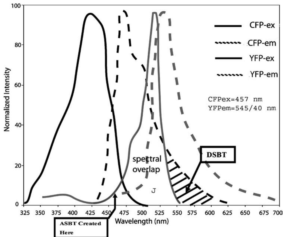
**Fig. 1.** Absorption and emission spectra of eCFP and eYFP. The DSBT area in the eYFP emission channel represents the donor spectral bleedthrough in the FRET channel and the arrow shows the donor excitation wavelength (457 nm) exciting acceptor molecule to cause acceptor bleedthrough.
